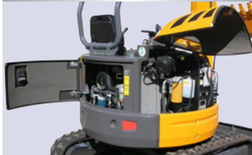
Hydraulic tank with air breather
