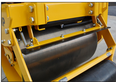
Spring loaded scraper bar folds up for easy change out and cleanup.
